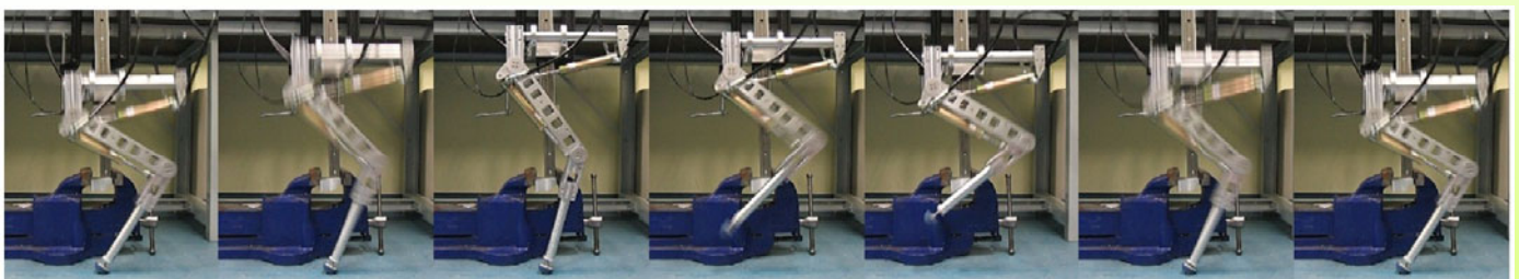
Picture sequence of the HyQ leg prototype clamped to the vertical slider test bench, performing a vertical jump motion. Time between two frames: 0.16 seconds.
